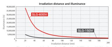
\*Measured value at an each given distance from the fiber exit face of 1,000 mm long straight light guide (with 8 mm bundle diameter) at maximum illuminance ( not guaranteed )
