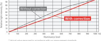
\* Actual value measured in accordance with our measurement standards \* Linearity correction function is always effective
