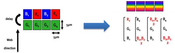
This colour mode ( $5\mu m$ ) requires the indication of "Forward/Reverse" to the camera in order to manage the delay between the two coloured lines.
