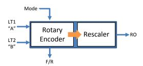
The Output of the Rotary Encoder enters a Rescaler (Multiplier / Divider) that can be also bypassed (neutral). The Rotary encoder has two working modes:
