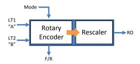
The Output of the Rotary Encoder enters a Rescaler (Multiplier / Divider) that can be also bypassed (neutral).
